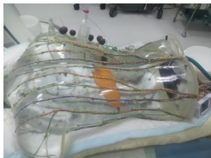
Torso tank set up, and set of active electrodes for EIT
