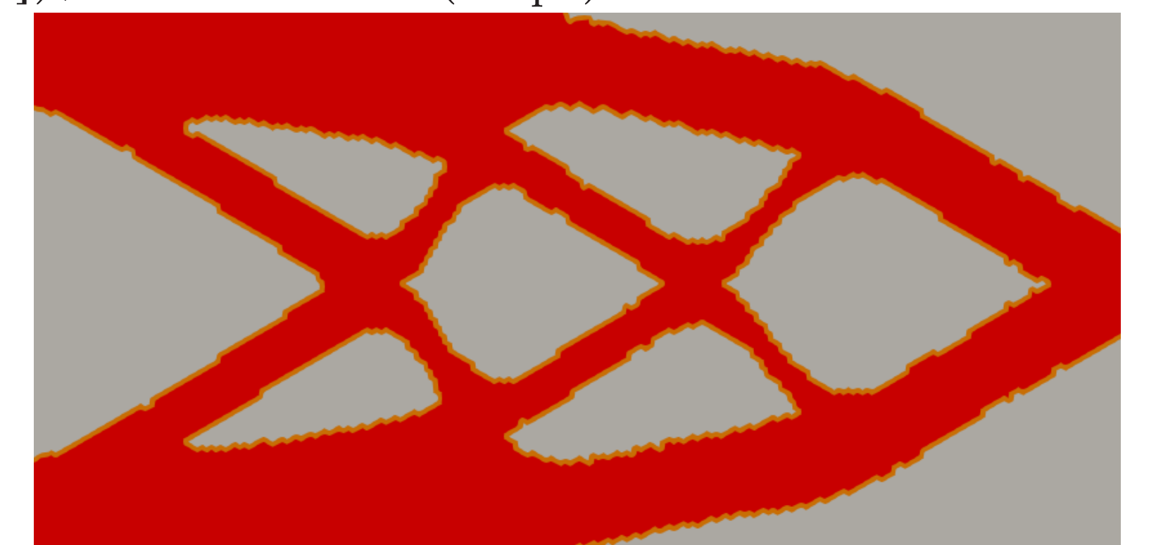
Fig. 3: Result of the shape optimization.
